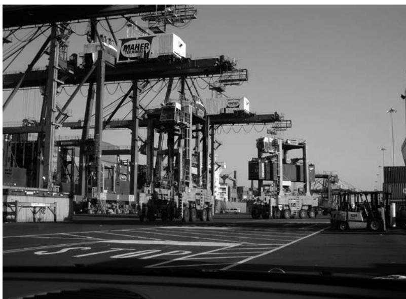
FIGURE 22. Gantry cranes in the Port of Elizabeth, New Jersey, 2006. Source: Photograph by the author.
